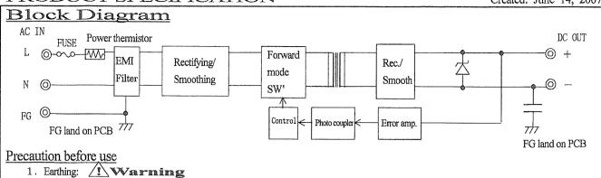
This power supply is designed and produced as Class I equipment. Make sure to securely connect earthing terminal (FG) to the ground in a proper way before use.
