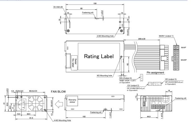
\*1 Dimensional tolerance shall be ± 1mm unless otherwise specified.
