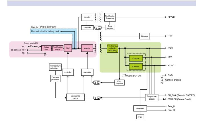
(1) Only +5VSB output starts up by supplying AC input while PS\_ON# is "H" status.
