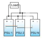
■Parallel connecting diagram for block terminal type
