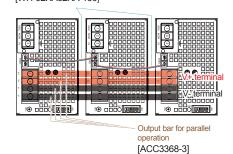
As in above picture, connect each output terminal with ACC3368-3 and each B.SIG terminal with WH-02XA02XA-150.
