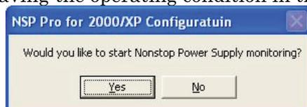
If Nonstop power supply monitoring is ready to start, click [Yes] button to start Nonstop power supply monitoring service. If not ready yet, click on [No] button. In either case, operating condition setup tool quits.
