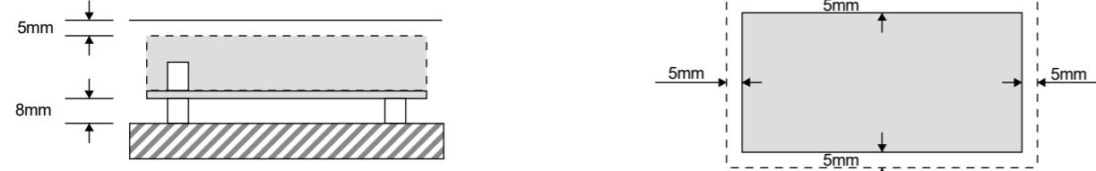
To suppress temperature rise around power supply, pay attention to set up to avoid poor convection or ventilation.
